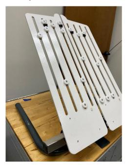
4. To set it up for production, you can move the white washers around by loosening the 4mm allen screw in the middle. Then position them so they will hold the outer ring of your hoop in place.
